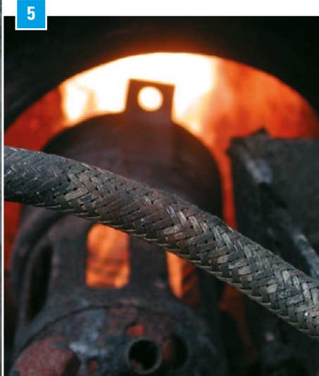
Pre-heating the special aggregate to 180 °C
