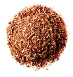
Dry, pourable ceiling infill. Dry earth fill material consists of clay and numerous softwood chips.
